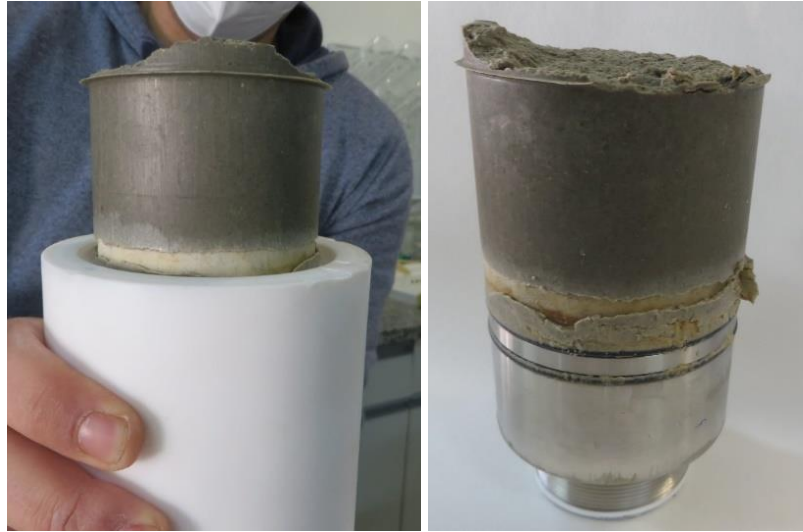
Figure 36 Upper part of the column corresponding to sampling sections S2 to S0 (upside down). Porous stone and material extruded upwards can be seen at the bottom of the photos
