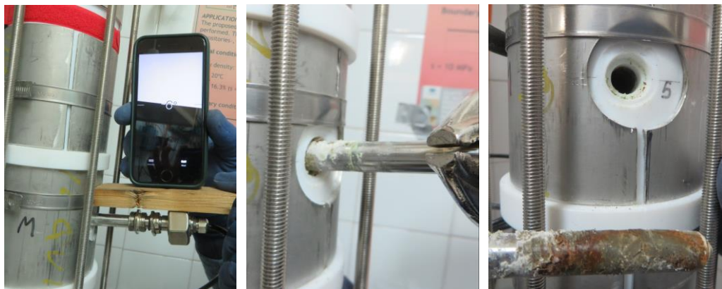
Figure 26 Sequence of extraction of sensor RH/T2
