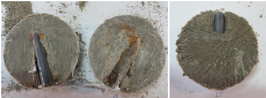
Figure 37 Retrieval of Teflon plugs inserted at the location of sensors RH/T2 (left) and RH/T1 (right)
