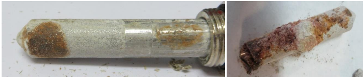
Figure 41 Appearance of the porous filter of sensors RH/T2 (left) and RH/T3 (right) after extraction
