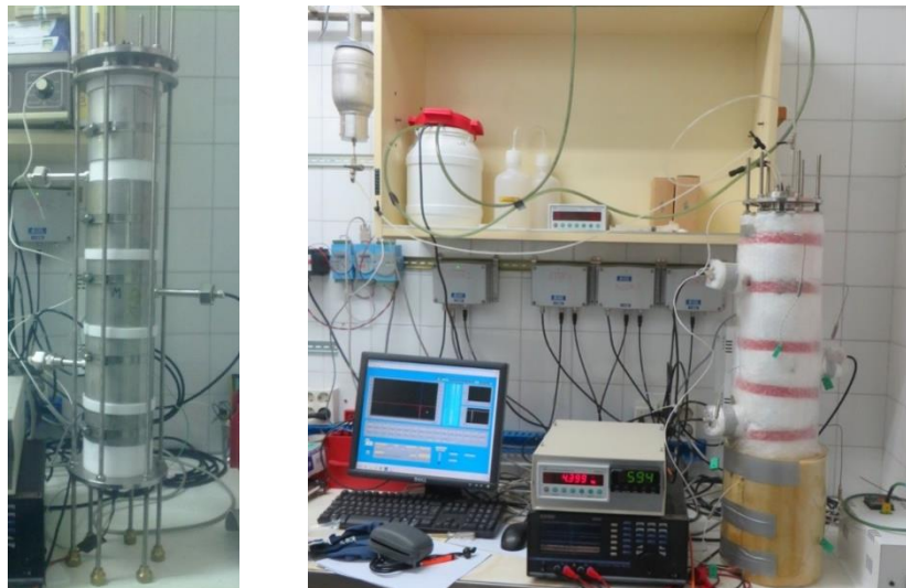
Figure 9 Cell B before being wrapped with the insulating material and during operation with the external insulation material
