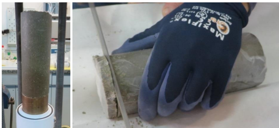
Figure 35 Extraction and sampling of the part of the column corresponding to sections S12 to S2
