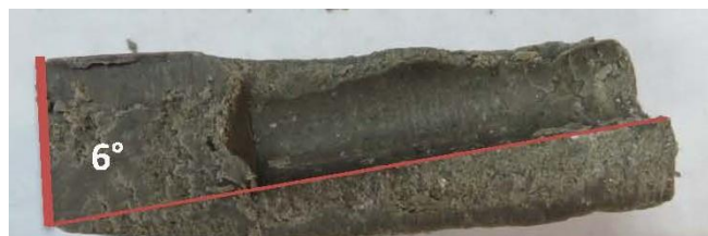
Figure 42 Mould in the bentonite of sensor RH/T1 showing its pitch
