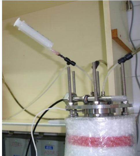
Figure 16 Hydration system with syringe connected for extracting air bubbles
