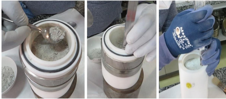
Figure 33 Subsampling of loose sections S25 to S20 and measurement of sampling sections height
